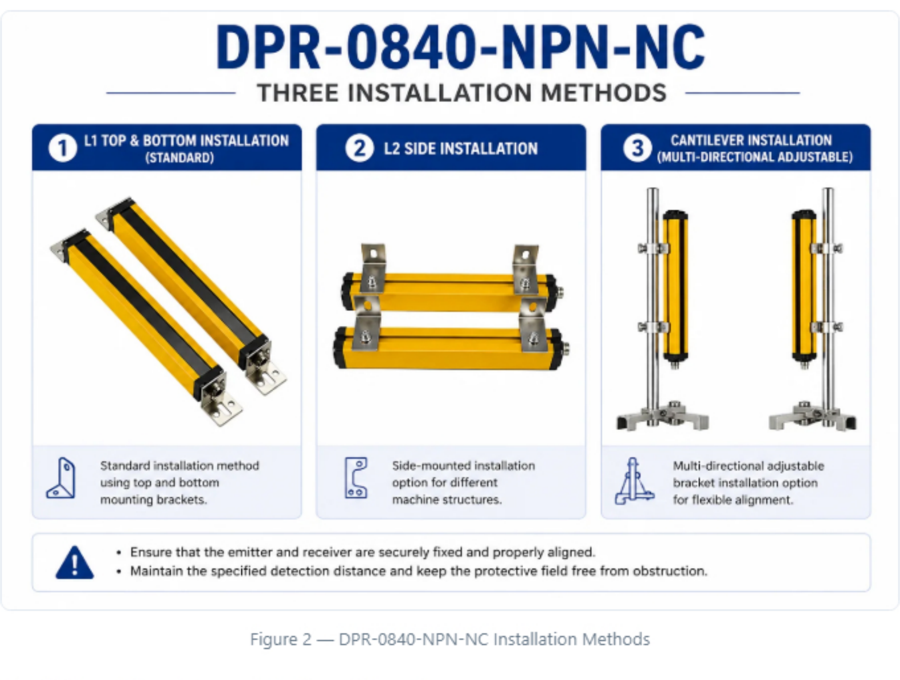
Figure 2 — DPR-0840-NPN-NC Installation Methods
