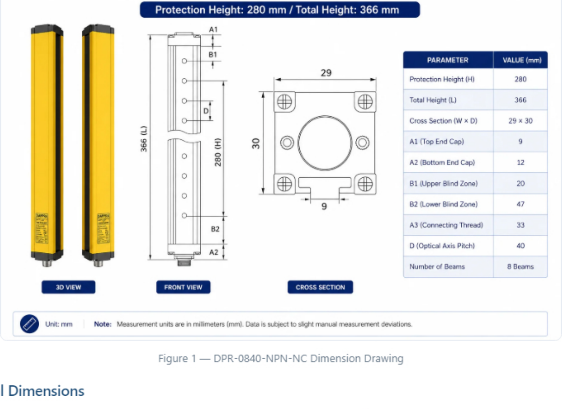
Figure 1 — DPR-0840-NPN-NC Dimension Drawing
